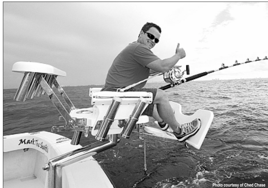
Quartiano's boat is equipped with a Lee's Fighting Chair, which extends out over the back end of the boat.
